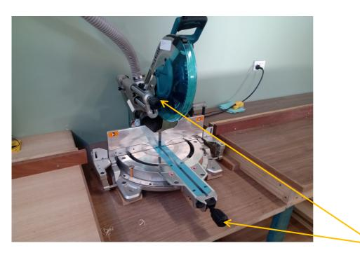
One of the two identical drop saws at LMCS, note the locking handles for the mitre and bevel adjustments.
