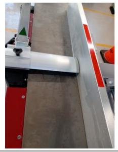
Hammer combination planer/thicknesser in planing mode. Note red zone on fence for location of fingers and green arrow for feed-in direction.
