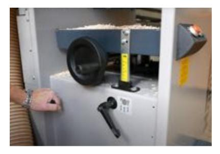
Planer-thicknesser in thicknessing mode. Note the feed-in engagement lever held by the operator's left hand.
