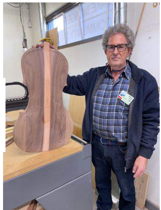
Final products after CNC....back and soundboard.
